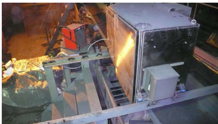
Figure 1. Laser analyzer installed at NLMK
